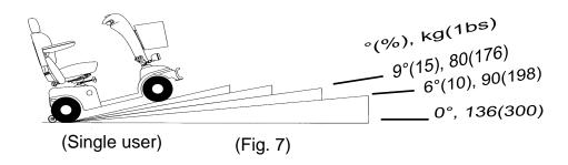
Angles and weights shown here for this scooter indicate the safe working angles for the user and equipment. Any scooter used outside these parameters may be unsafe and or cause future problems with the electrical systems
