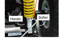
Remark: Please do not twist counterclockwise from the position No.5 next to No.1 as shown, otherwise, it's no way to reverse from position No.1 back to No.5 unless to take apart the whole suspension assembly from the rear chassis to reset the standard position of the adjustablesuspension assembly.
