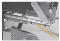
When changing the position of the back rest hinge, also remember to change the position of the gas strut under the chair. The bracket has 3 holes. When the back rest hinge is set in the shortest position, the gas spring is placed in the front hole using the short locking head.
