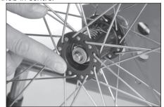
To check that the drive wheel is properly attached to the hub, remove the finger from the central knob and pull the main wheel.
