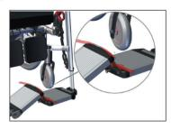
While making the adjustment, there must be no load on the foot plates.
