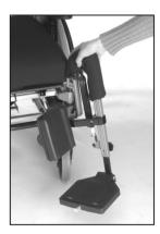
▲ When adjusting leg support angle, be aware of squeeze hazard between moving parts.
